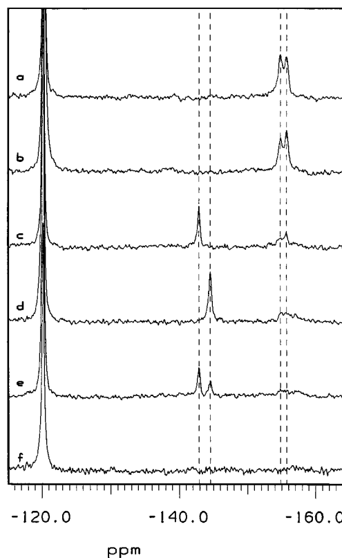
FIGURE 2: 19 F NMR spectra of Rho·GDP and RhoGAP in the presence of AlCl 3 and NaF. All 19 F NMR spectra were recorded in buffer containing 50 mM Tris/HCl, pH 7.5, 5 mM NaF, 1 mM AlCl 3 , 1 mM MgCl 2 , and 5% D 2 O. Spectra were recorded in the absence of protein (a), after addition of 200 μM Rho·GDP (b), and following subsequent addition of 200 μM wild-type RhoGAP (c). In a separate experiment, 200 μM Rho·GDP and 200 μM mutant R282A RhoGAP were mixed (d) followed by addition of 166 μM wild-type RhoGAP (e). After recording spectrum c in the presence of Rho·GDP and wild-type RhoGAP, 2.5 mM deferoxamine was added and the spectrum re-recorded (f). For spectra a–e 3000 scans and for spectrum f 1666 scans were acquired. The spectra are scaled accordingly.
